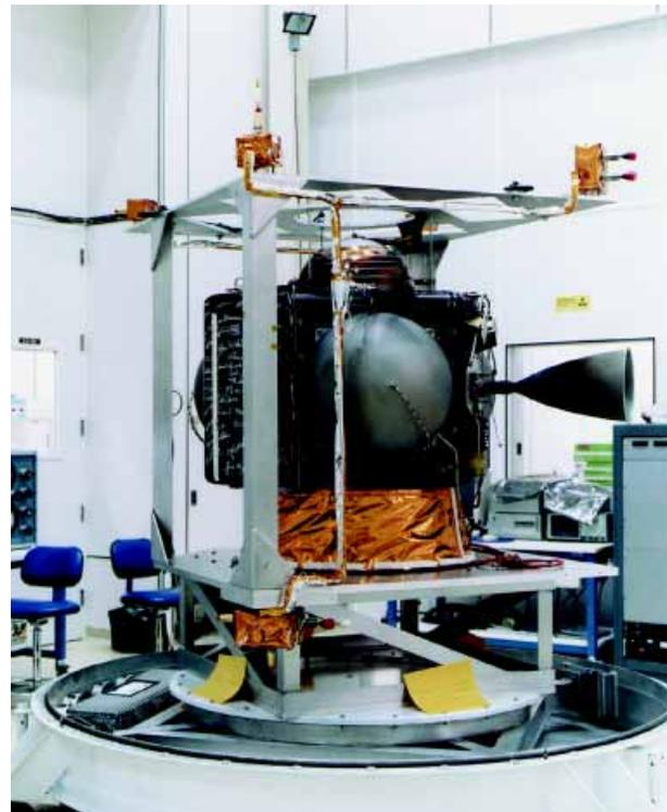
**Figure 1.** The propulsion subsystem in its shipping frame before spacecraft integration. Note that the large velocity adjustment thruster is mounted horizontally. The fuel and oxidizer tanks are mounted symmetrically with respect to the thrust axis to maintain the thrust vector through the spacecraft's center of gravity during fuel depletion.
