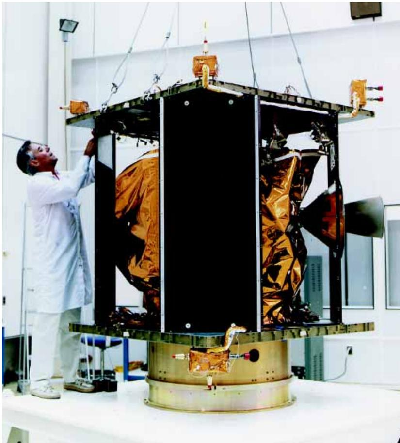
**Figure 2.** The completed structural assembly with the four fixed side panels installed. The four removable side panels are not installed to allow access inside the spacecraft structure.
