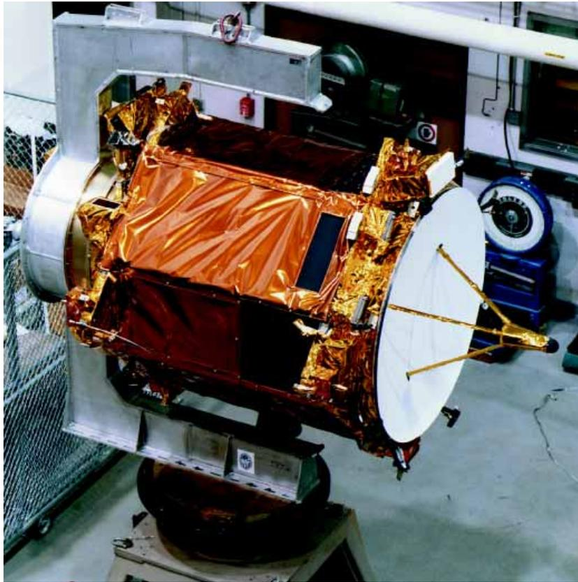
**Figure 5.** The spacecraft with solar panels removed and mounted on the turnover yoke for horizontal mass properties measurements at Goddard Space Flight Center.
