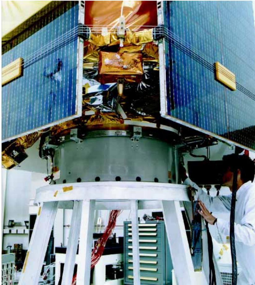
**Figure 4.** The flight despin system. The two despin cables were each wrapped twice around the spacecraft, guided by the combs mounted on the solar panel edges. Foam pads were positioned between the cables and the solar cells to prevent cell damage during vibration.
