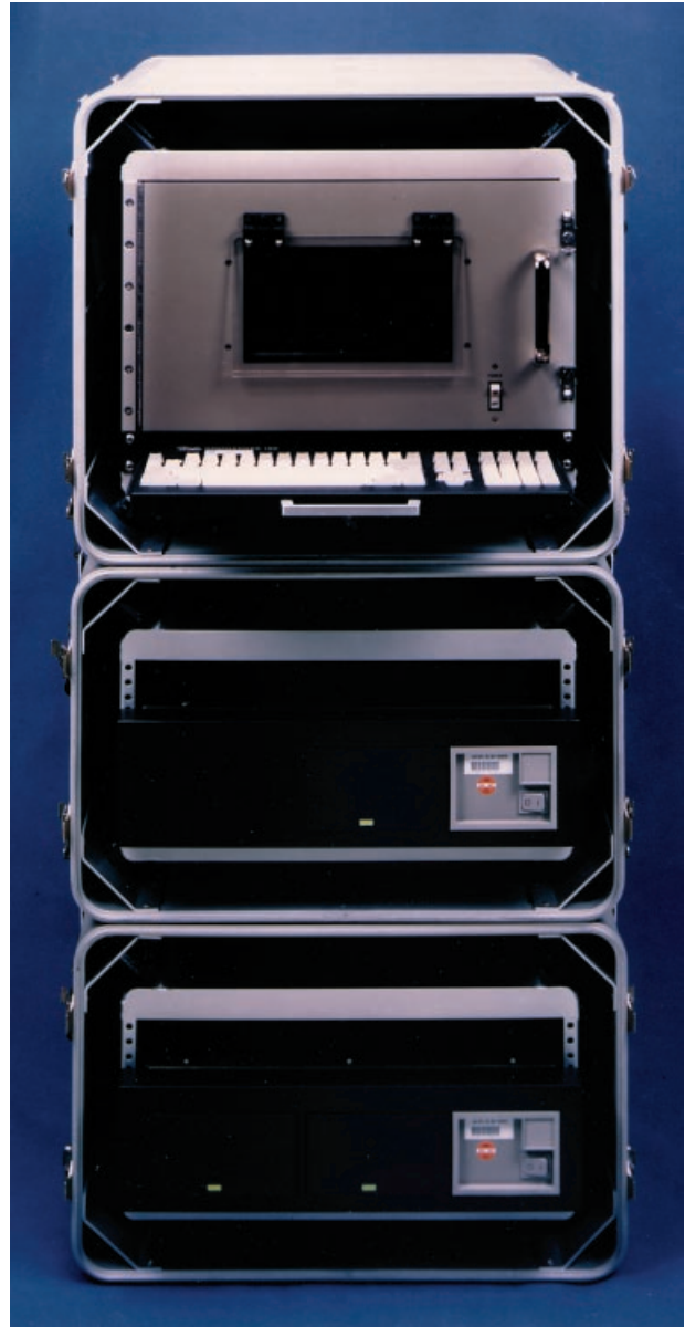
Figure 4. Parallel disk array, keyboard, and monitor screen housed in shock-mounted enclosures. This configuration was originally designed for use aboard a target ship, where sonic booms and generally rough operating conditions make it necessary to protect the hard disk drives from excessive shock. This system can store up to 2.6 GB of data at up to 8 MB/s. It has been used with the Phalanx coherent data collector (CDC), the AN/SPS-48E CDC, and the AN/SPS-48E auxiliary detection processor.
