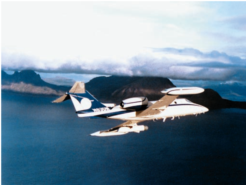
Figure 1. The Captive Seeker wing pod is shown mounted on a Flight International Learjet. This photograph was taken during initial testing to characterize land backscatter in Vestfjord, Norway.
