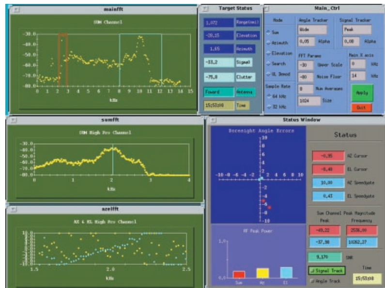
Figure 6. Captive Seeker System spectral analysis display. Doppler frequency spectra allow the operator to see what a Standard Missile will process in terminal homing. The display also serves as the means to input signal and angle track parameters.
