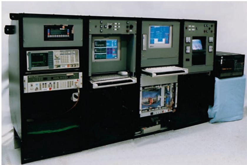
Figure 3. Captive Seeker cabin-mounted electronics. These racks were designed at APL to conform to the Learjet interior while providing standard rack-mounting surfaces for commercial and APL-designed equipment.
