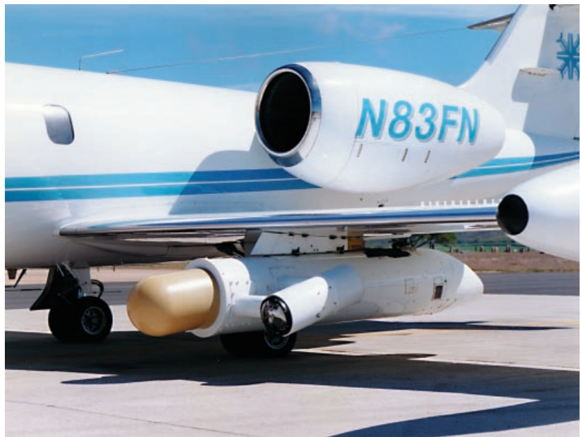
Figure 2. Close-up of the Captive Seeker wing pod. The steerable RF antenna is mounted behind the radome. A boresighted video camera is mounted in the smaller, slightly slanted tube.
