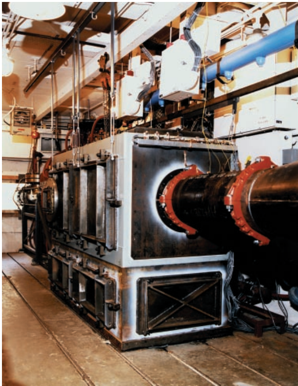
Figure 4. Supersonic wind tunnel capable of performing Mach 4–7 freejet engine tests.
