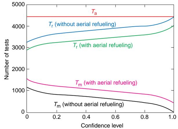
**Figure 2.** F/A-18 E/F flight test scheduling margin.  $T_a$  = overall number of available test windows,  $T_r$  = overall number of required test windows, and  $T_m$  = available scheduling margin.
