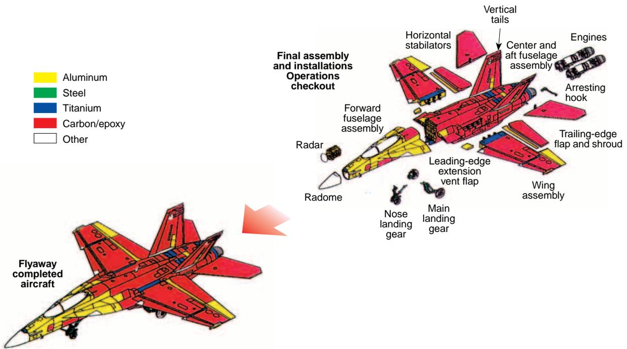
**Figure 5.** Composite materials will comprise 19% of the structural weight and 60% of the external surface area of the F/A-18 E/F aircraft.
