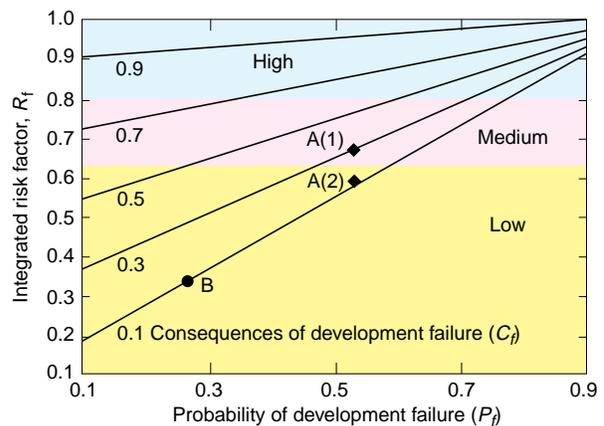
**Figure 4.** Integrated risk factor plotted as function of  $P_f$  and  $C_f$ .
