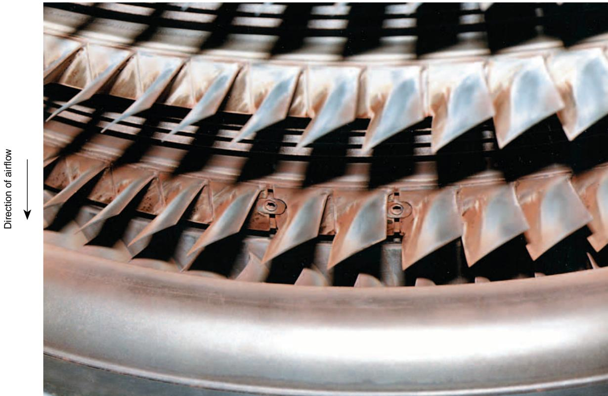
**Figure 6.** Potassium phosphate deposits on sixth and seventh stage blades of the F414 compressor .
