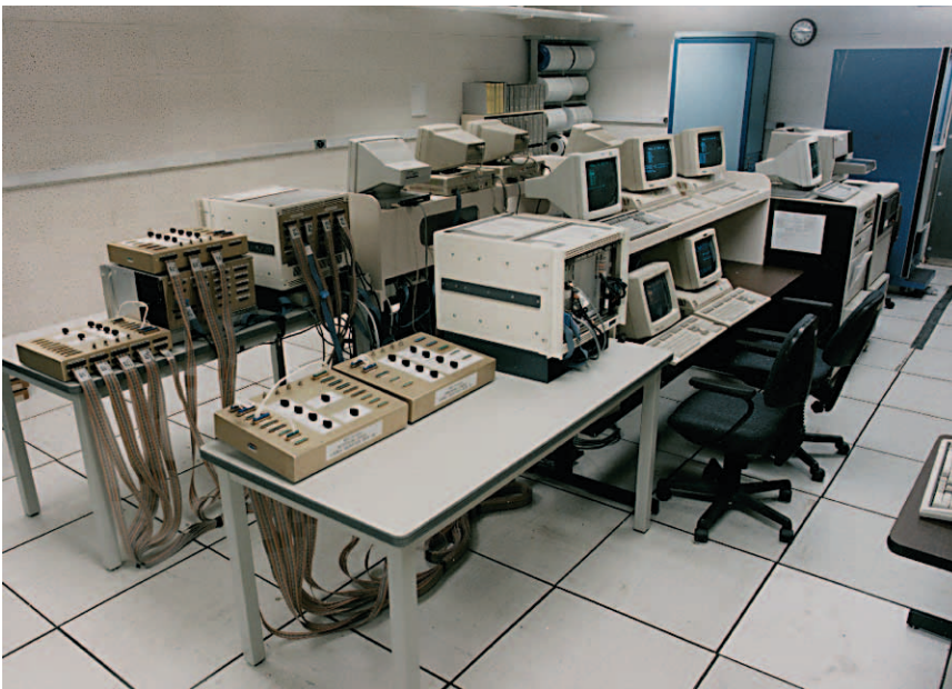
Figure 4. Testbed simulator laboratory. The two identical copies of the testbed are arranged back-to-back in this view. From foreground to background, the visible elements of the testbed are the two cable adapter boxes, the VMEbus chassis, display terminals, and MicroVAX computer cabinets.
