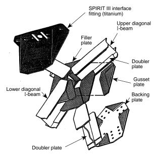
Figure 7. SPIRIT III interface fitting. All components are G/E unless noted.
