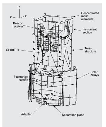
Figure 9. MSX launch configuration finite element model.
