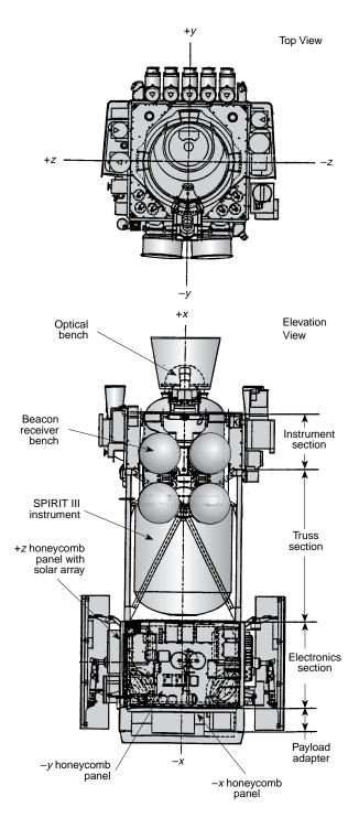
Figure 2. The MSX spacecraft configuration (stowed).
