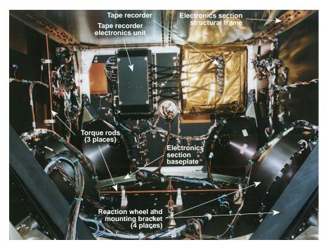
Figure 3. Interior of the electronics section.
