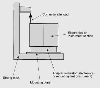
Figure 10. Static load test set-up: corner fittings.
