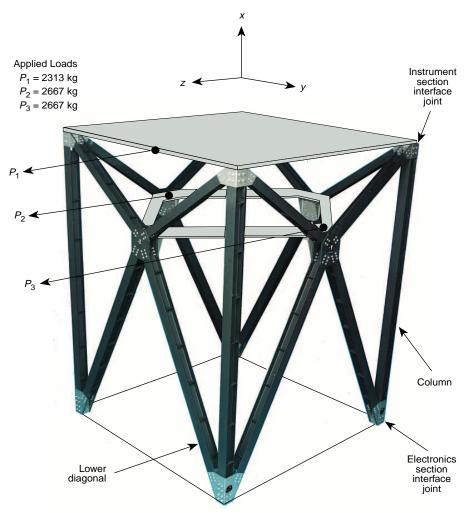
Figure 12. Truss structure static load test set-up.
