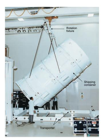
Figure 15. MSX shipping container and lift/rotation fixture.
