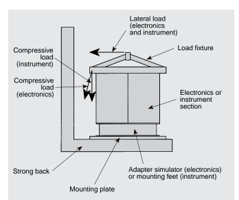
Figure 11. Static load test set-up: overall structural integrity.
