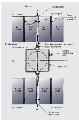
Figure 4. MSX solar arrays: deployed configuration. Arrays are rotated with the panel "cell side" shown. INBD, inboard; OTBD, outboard; Quad, quadrant.
