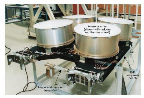
Figure 14. MSX beacon receiver subsystem.
