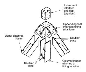
Figure 8. Upper diagonal interface fitting. All components are G/E unless noted.
