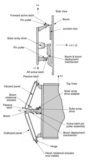
Figure 5. MSX solar arrays: stowed configuration.
