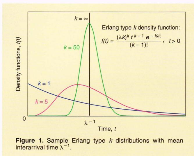
**Figure 1.** Sample Erlang type  $k$  distributions with mean interarrival time  $\lambda^{-1}$ .
