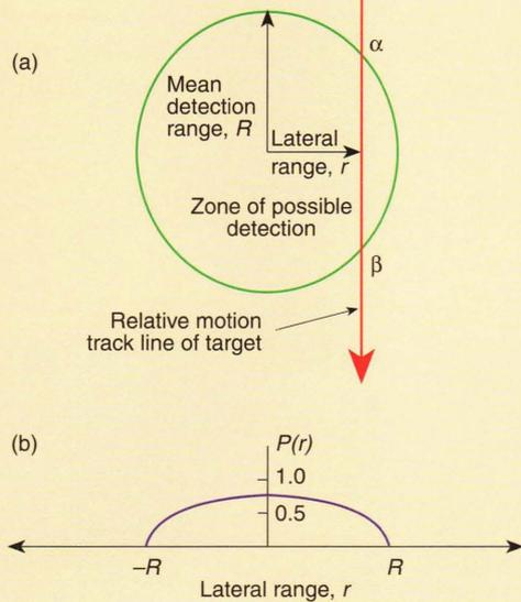
**Figure 3.** For a particular sensor environment, a lateral range curve represents a target's cumulative probability  $P$  of being detected as a function of its lateral range  $r$ . (a) Lateral range geometry, where  $\alpha$  is the point at which the target enters the zone of possible detection and  $\beta$  is its point of departure. (b) Hypothetical lateral range probability curve.
