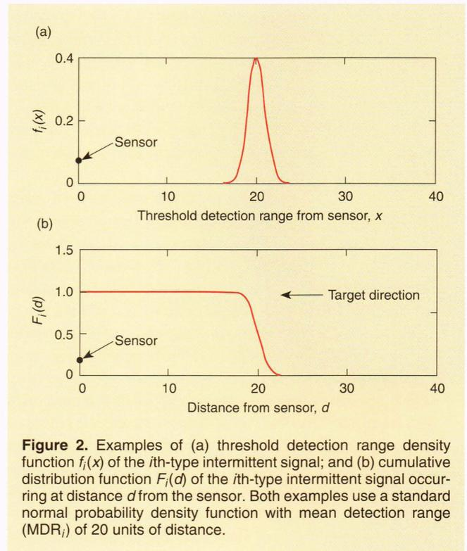
**Figure 2.** Examples of (a) threshold detection range density function  $f_i(x)$  of the  $i$ th-type intermittent signal; and (b) cumulative distribution function  $F_i(d)$  of the  $i$ th-type intermittent signal occurring at distance  $d$  from the sensor. Both examples use a standard normal probability density function with mean detection range ( $\text{MDR}_i$ ) of 20 units of distance.
