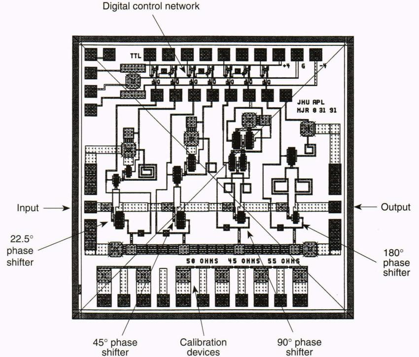
**Figure 6.** Computer-generated drawing of phase shifter layout showing four cascaded phase-shifter elements and supporting digital bias generating network.
