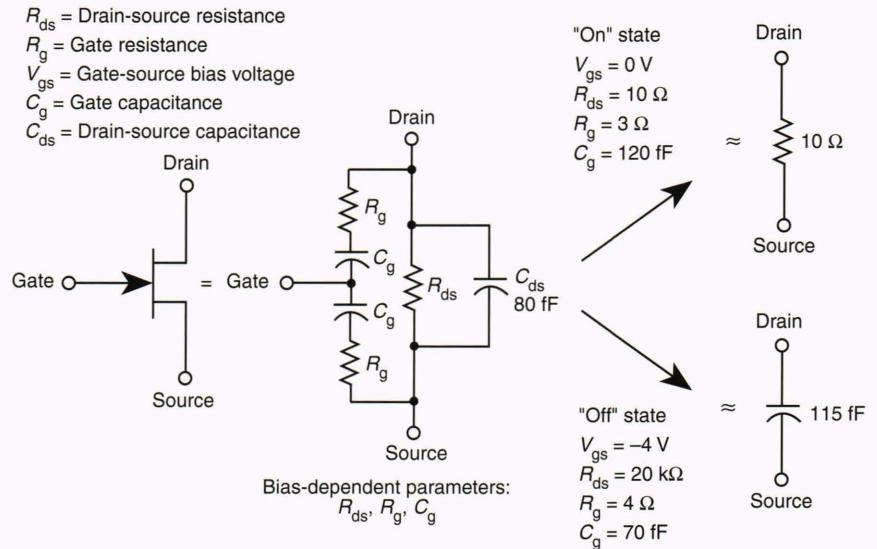
**Figure 3.** Field-effect transistor (FET) electrical switch model. An FET can be used in a switch mode by altering the gate bias voltage to place the device in a high-conductance "on" state or in a pinched "off" state. The values shown represent a 300- $\mu\text{m}$  FET. The simplified electrical model reduces to a resistor for the "on" state and a capacitor for the "off" state.
