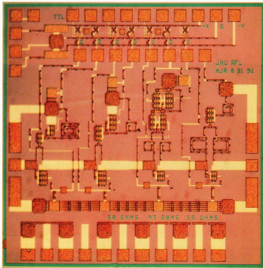
**Figure 8.** Microphotograph of fabricated phase shifter on gallium arsenide substrate. The circuit measures 0.09 by 0.09 in.
