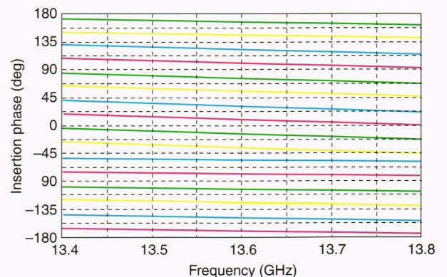
**Figure 7.** Computer-simulated insertion phase length versus frequency. Sixteen states are shown from  $-180^\circ$  to  $+180^\circ$  in increments of 22.5°. Phase change is defined as the relative difference between these states.
