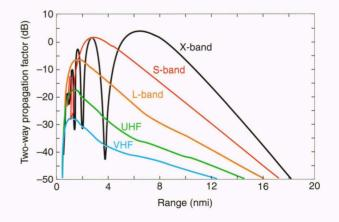
**Figure 9.** The low-elevation two-way propagation factor is shown for several frequencies at a radar antenna height of 100 ft for a seaskimming cruise missile at a 12-ft altitude. The X-band advantage over S- or L-band at a detection range of 10 nmi is as great as 16 or 27 dB, respectively.
