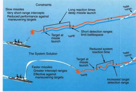
Figure 3. Projected combat system challenges in engaging advanced supersonic sea-skimming cruise missiles include short detection ranges, long reaction times, and defensive missiles with reduced performance against advanced, highly maneuvering threats. Effective defense requires detection, command and control, hardkill and softkill system enhancements, and increased system automation and integration.
