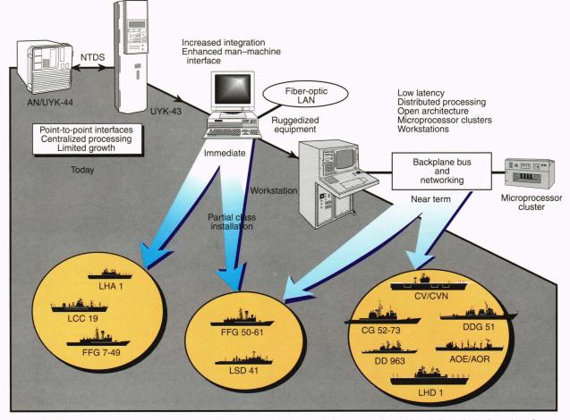
**Figure 13.** The system requirements allocated to the command and control element can be achieved through the insertion of current technology in computer processing, networking, and displays. Increased integration, data fusion, distributed-microprocessor-based processing, and enhanced man-machine interfaces enable rapid-response, low-data-latency weapon system operations. Ship class descriptions can be found in Ref. 11. NTDS = Naval Tactical Data System, LAN = local area network.
