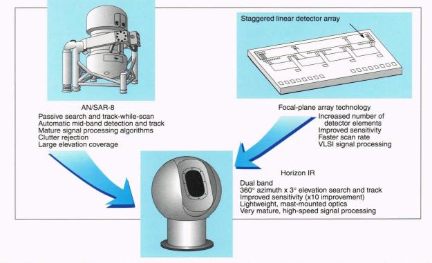
Figure 11. Engagement battlespace lost owing to the high-speed, low-altitude, and small radar-cross-section supersonic cruise missile can be regained through multispectral data fusion and radar cueing using focal-plane-array IR sensor technology with improved sensitivity and a faster scan rate. Lightweight optics permit high mast mounting, which further extends the horizon and detection range against the high-speed (thus "hot" IR signature) threat. VLSI = very large scale integrated circuit.
