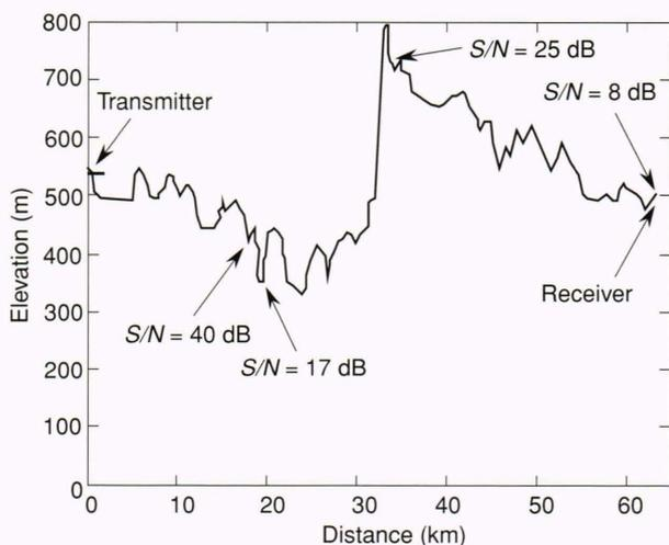
**Figure 6.** Terrain profile for path 1 into the Schwäbian Alps shown in Figure 5. S/N = signal-plus-noise to noise ratio.
