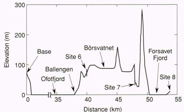
**Figure 12.** Terrain profile for the high-frequency ground wave path from base to sites 6, 7, and 8 in Norway. The path crosses the Ofotfjord Fjord, Börsvatnet Lake, and Forsavet Fjord.
