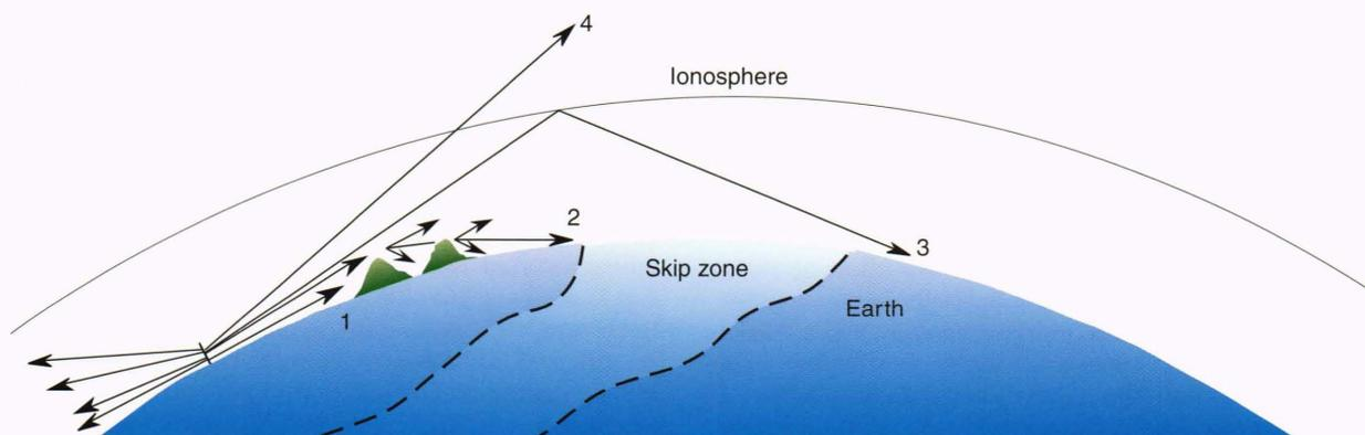
**Figure 1.** Radiation emitted from an antenna on the Earth's surface. Ray 1, wave glides along interface between air and ground; ray 2, wave travels directly to distant mountain and diffracts from mountain peak; ray 3, wave travels into sky, interacts with ionosphere, and reflects back to a distant point; ray 4, wave passes through the ionosphere and into space. No wave is present in the skip zone.
