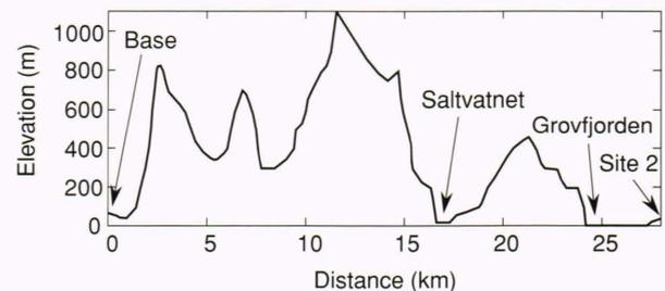
**Figure 9.** Terrain profile for the high-frequency ground wave path from base to site 2 near Fornes, Norway. The path crosses Saltvatnet Lake and Grovfjorden Fjord.
