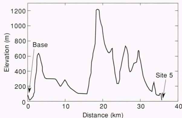
**Figure 11.** Terrain profile for the attempted high-frequency ground wave (HFGW) path from base to site 5 near Sandstrand, Norway. No HFGW communications could be established over this path.
