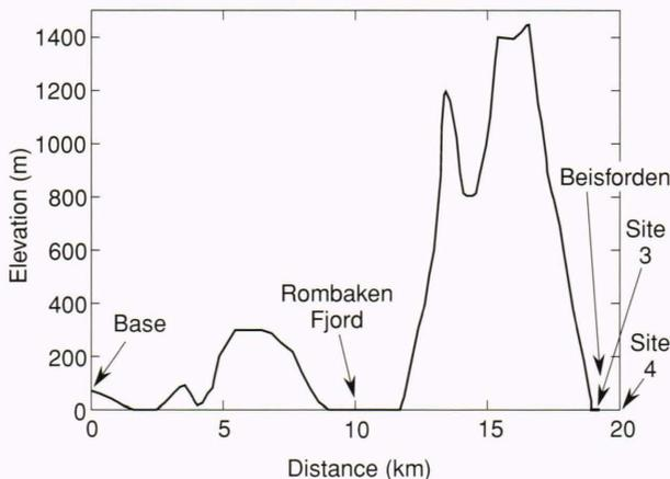
**Figure 10.** Terrain profile for the high-frequency ground wave path from base to sites 3 and 4 in Norway. Signal measurements were made from a boat on Beisfjorden Fjord.
