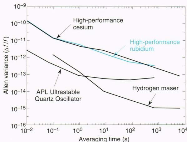
**Figure 2.** Frequency stability of a modern APL satellite oscillator in terms of Allen variance versus averaging time. Over certain important regions of operation, the APL quartz oscillator compares favorably with more complex oscillators ( $f$  = frequency).
