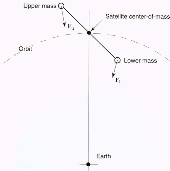
**Figure 5.** The gravity-gradient concept. The attractive force ( $F_l$ ) on the lower mass  $m$  of a barbell-shaped satellite exceeds the attractive force ( $F_u$ ) on the upper mass. A torque, therefore, arises to align the satellite toward the vertical.
