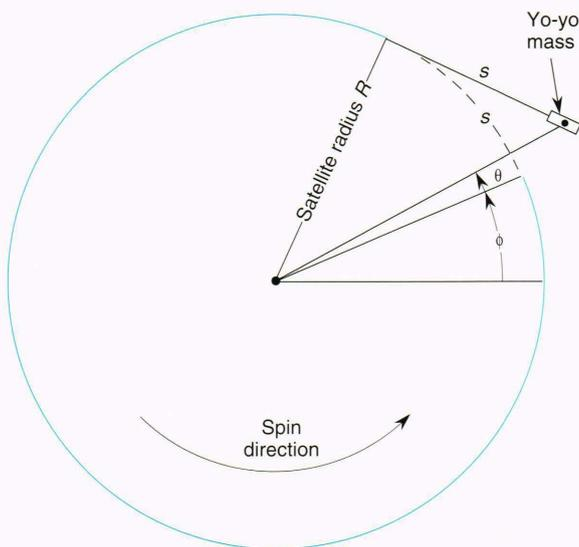
**Figure 4.** Yo-yo geometry showing the variables used in Equations 3 and 4, which describe the removal of spin by deploying a yo-yo on a wire ( $s$  = amount of wire paid out,  $\phi$  = angle turned by the satellite after release of the weight, and  $\phi + \theta$  = the polar coordinate of the weight).
