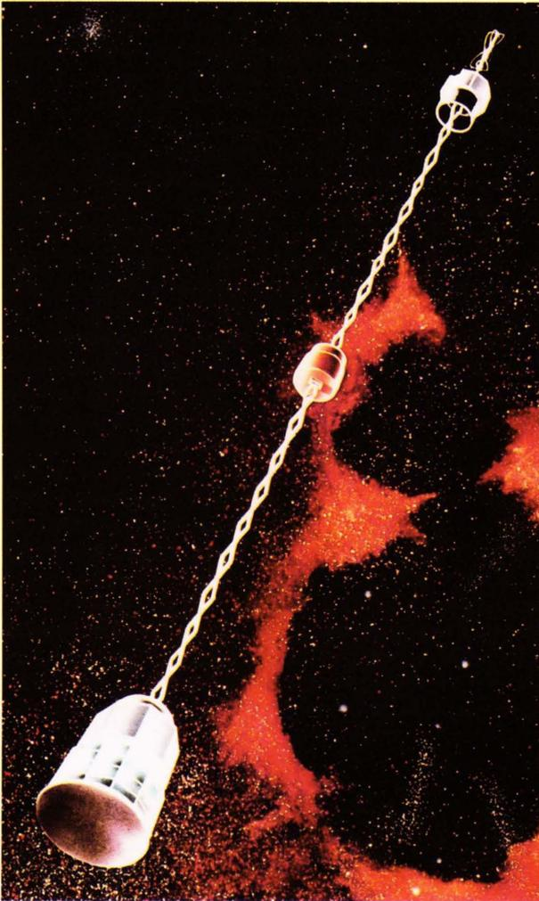
**Figure 7.** The first drag-free satellite, Triad. The central unit contains the DISCOS (Disturbance Compensation Device). The Earth-pointing portion (bottom) carries nested quadrifilar helix antennas. The top unit contains the nuclear power supply, the last of six flown by APL.
