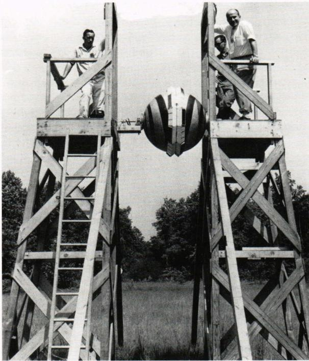
**Figure 3.** The yo-yo mechanism being tested on APL's first satellite, Transit 1-A. Logarithmic spiral antennas are painted on each hemisphere. James F. Smola (right) is now Spacecraft Manager of APL's fifty-fifth satellite, the MSX (Mid-Course Space Experiment).
