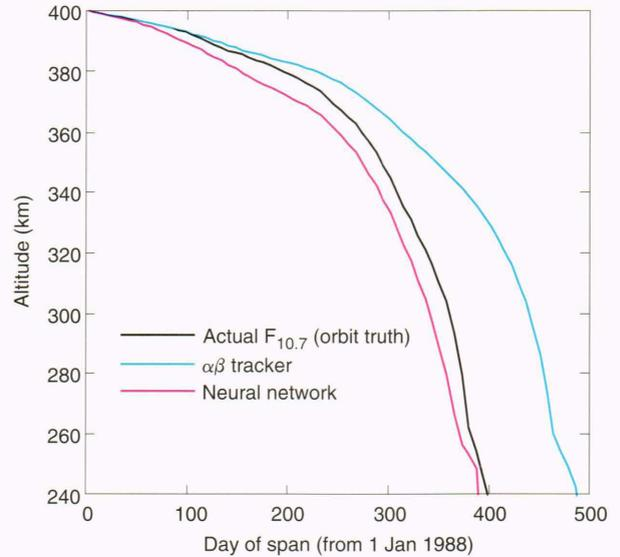
**Figure 10.** A comparison of orbit lifetimes based on different prediction methods with those based on actual solar data for an object similar to space station *Freedom* (area-to-mass ratio =  $4.54 \times 10^{-3} \text{ m}^2/\text{kg}^{-1}$ ; coefficient of drag = 2.2).
