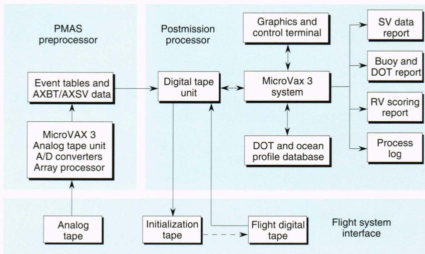
**Figure 11.** Postmission analysis system (PMAS) block diagram (RV = reentry vehicle, DOT = deep ocean transponder, A/D = analog-to-digital, AXBT/AXSV = aircraft-launched expendable bathythermograph/aircraft-launched sound velocimeter, SV = sound velocity).
