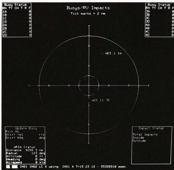
**Figure 10.** Display generated during “reseed” development tests where failed sonobuoys must be replaced (RV = reentry vehicle; ADI = air-deployable DOT interrogator).
