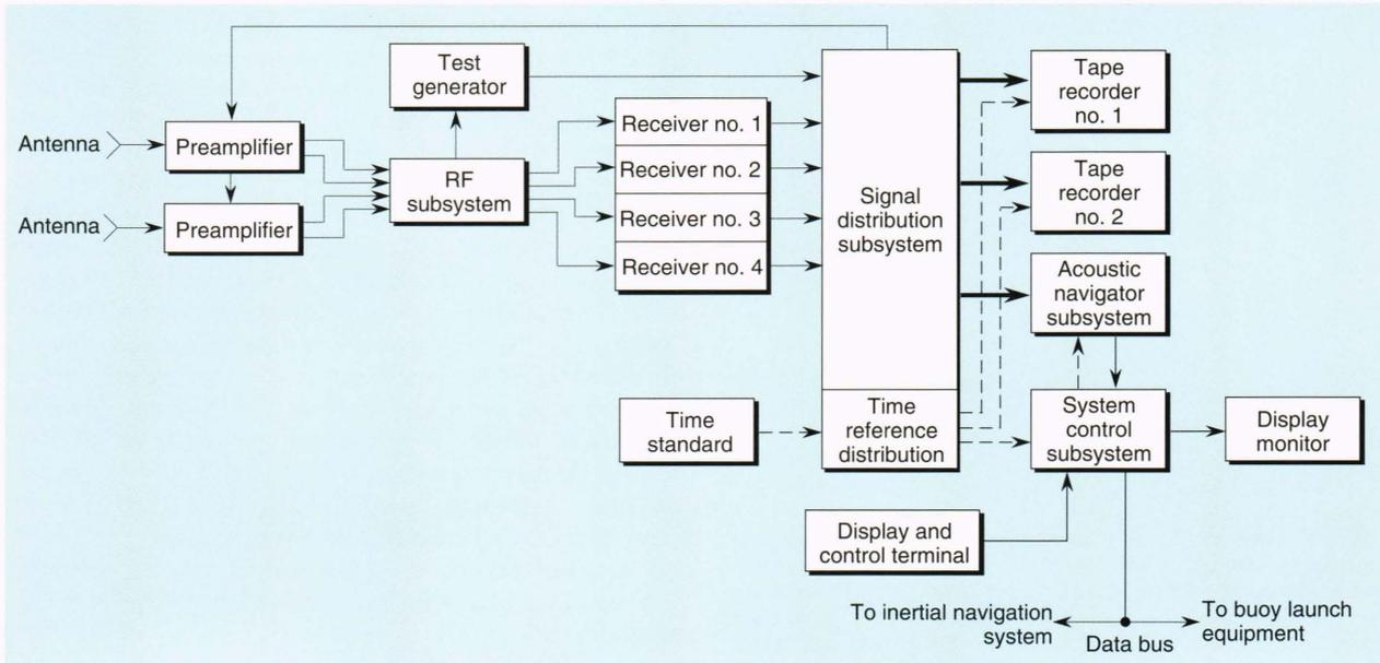
**Figure 6.** Block diagram of the Advanced Range Instrumentation Aircraft/Sonobuoy Missile Impact Locating System (ARIA/SMILS) Airborne Flight System.
