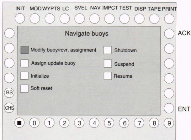
**Figure 9.** Example of menu and selection made by the operator during buoy navigation. The operator makes a selection by pressing the control next to the appropriate choice (INIT = initialize the menu; MOD = modify parameters menu; WYPTS = waypoints menu; SVEL = sound velocity menu; NAV = navigate buoys menu; IMPCT = impact location menu; DISP = display menu; TAPE = magnetic tape recorder menu; PRINT = printer menu; ACK = acknowledge message; ENT = enter; CHS = change sign; BS = back-space).
