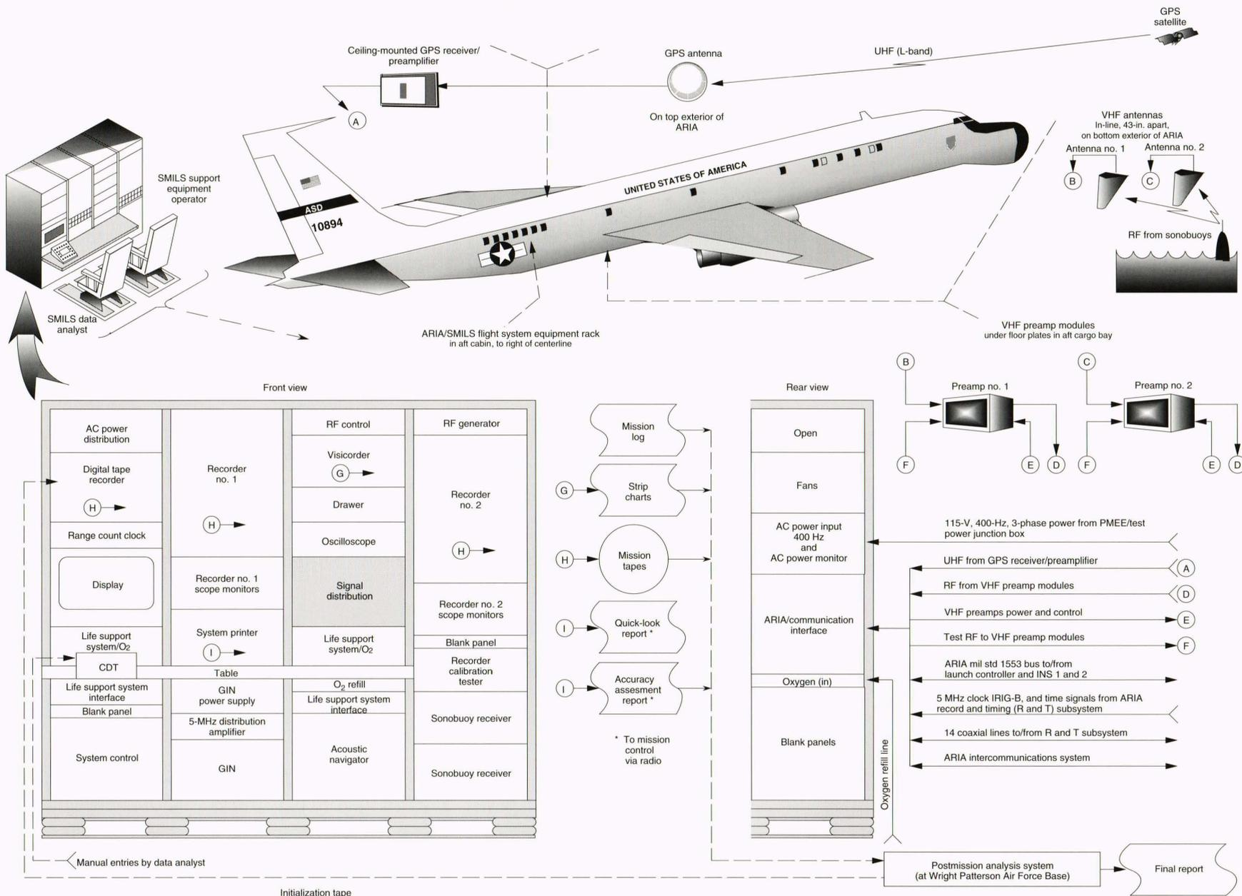
**Figure 4.** Illustration of the Sonobuoy Missile Impact Locating System (SMILS) equipment mounted inside the Advanced Range Instrumentation Aircraft (ARIA) (GPS = Global Positioning System, GIN = the GPS instrumentation navigator, CDT = the command and display terminal, IRIG-B = inter-range instrumentation group B, INS = inertial navigation system).
