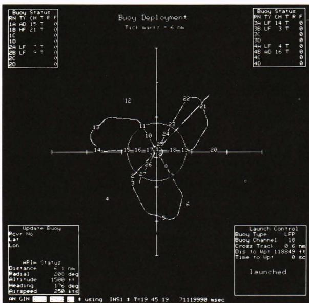
**Figure 7.** Aircraft track and buoy launch sequence as displayed by system control (LFP = low-frequency pinger, AN = acoustic navigator, GIN = Global Positioning System instrumentation navigator, INS = inertial navigator system, T = time, Wpt = waypoint).
