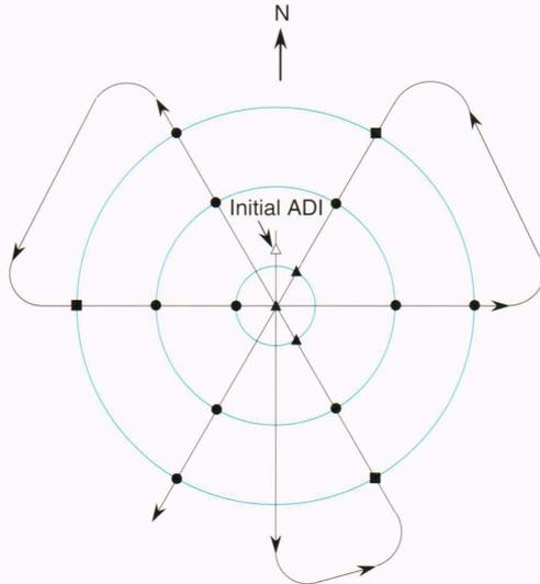
**Figure 5.** Nominal Advanced Range Instrumentation Aircraft/Sonobuoy Missile Impact Locating System (ARIA/SMILS) sonobuoy deployment pattern. Triangles indicate air-deployable interrogator (ADI); circles, low-frequency pingers; and squares, high-frequency buoys.
