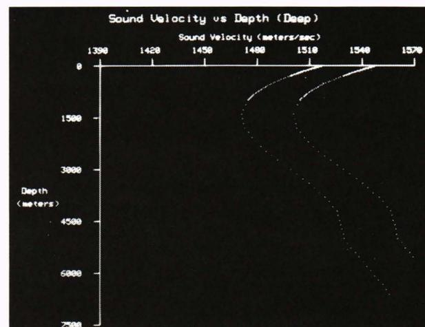
**Figure 8.** Sound velocity (SV) profile computed by the acoustic navigator and displayed by system control.
