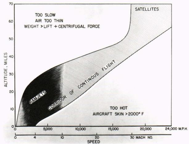
**Figure 13.** William H. Avery's televised talk suggested that ramjets would be able to fly more than thirty miles high at 10 times the speed of sound.
