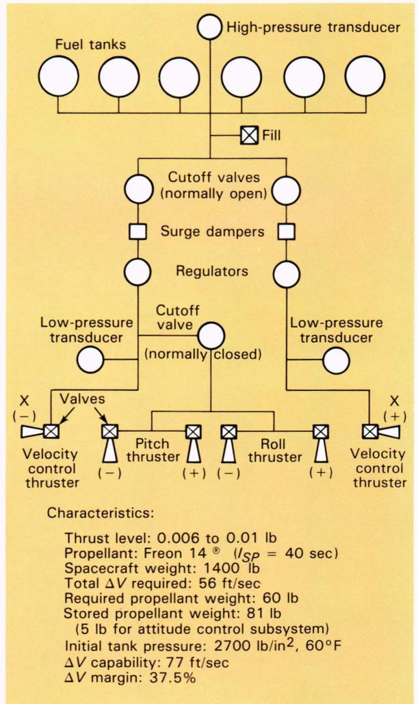
Figure 5—Schematic diagram of the velocity control system.
