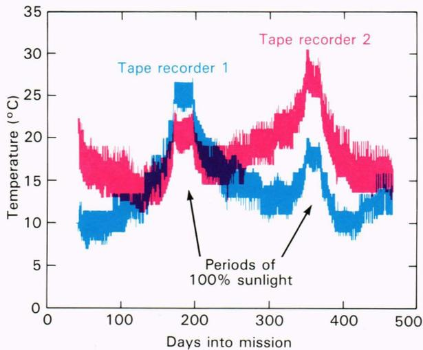
Figure 6—External temperatures of the tape recorders.
