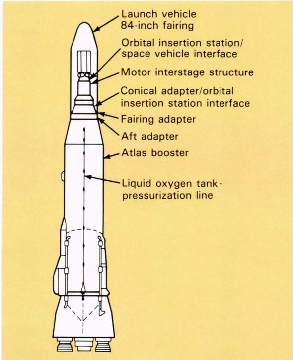
Figure 3—Launch vehicle configuration.
