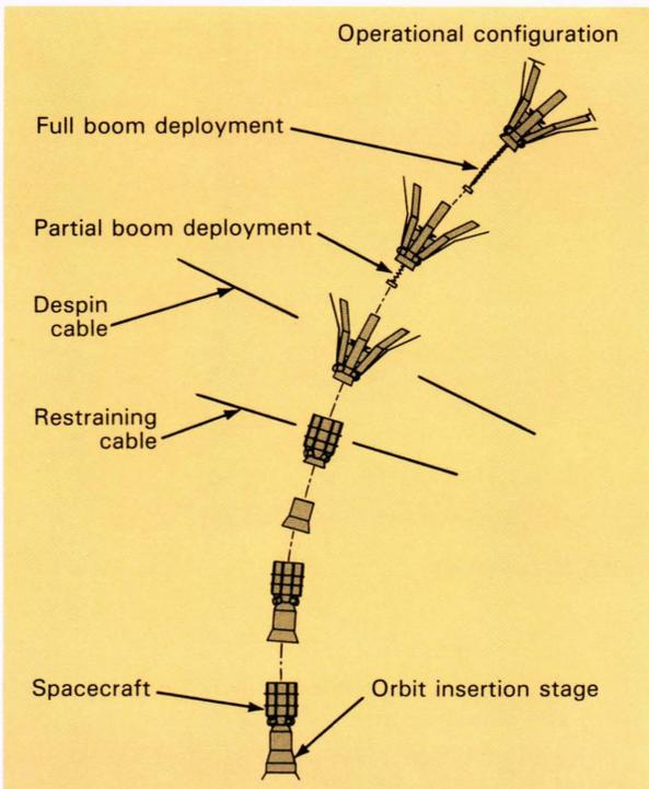
Figure 4—Orbit insertion phase.
