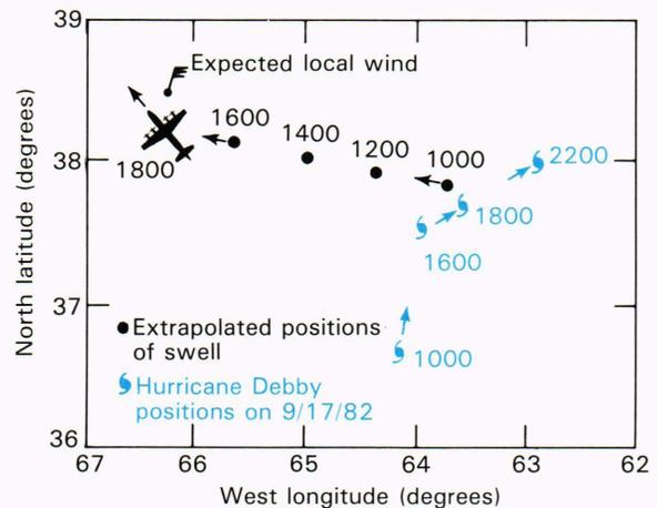
**Figure 9**—Plan view of the aircraft position and the Hurricane Debby ground track.
