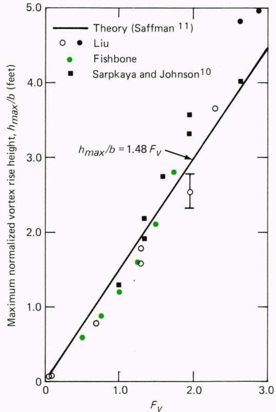
**Figure 14**—Maximum rise height of vortex pairs.
