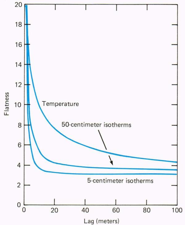
**Figure 8**—Lagged flatness computed for three series: isotherms calculated at 5 centimeters, isotherms calculated at 50 centimeters, and the temperature (75 kilometers of data averaged).
