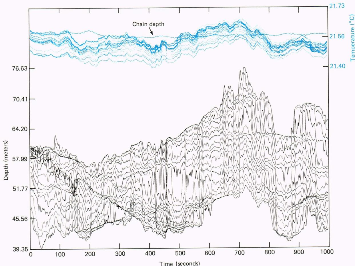
**Figure 5**—A representative segment of intercalibrated temperatures, plotted on the bottom half of the figure, and isotherms calculated from those temperatures, plotted on the top.
