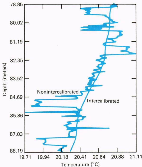
**Figure 1**—Vertical profile of temperature averaged over 50 meters horizontally. The smooth curve represents a calibrated profile.
