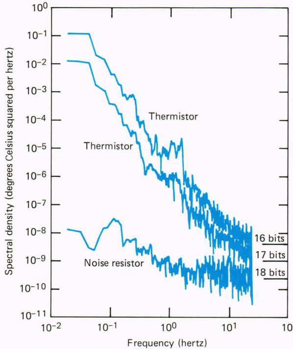
**Figure 6**—The autospectral density of two thermistors and the noise resistor from gradiometer 10. Equivalent bit noise levels are indicated on the right for a 20° operating range.
