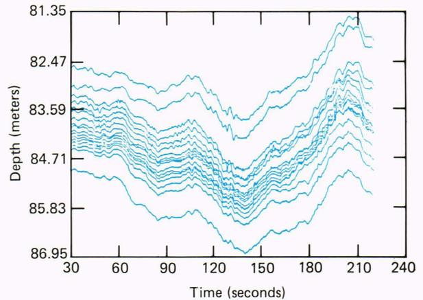
Figure 3—Modified inversion-avoiding composite isothermal displacements (MIACID). Note the lack of step-like structures.
