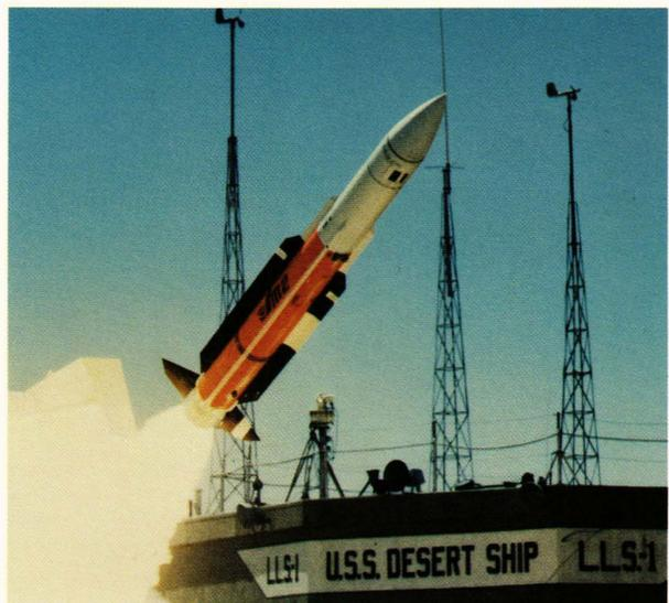
**Figure 9** — Launch of an AEGIS SM-2 flight test round at the USS DESERT SHIP at White Sands Missile Range.
