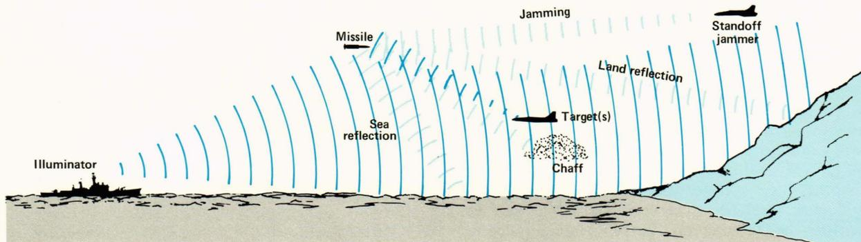
**Figure 4** — Typical signals received by the missile in flight. Good steering information can usually be derived from either target-reflected energy or jamming energy from the target. Interfering signals, which can exceed the target skin return by many orders of magnitude, must be rejected. Interference derives from natural and man-made environments, both friendly and unfriendly.
