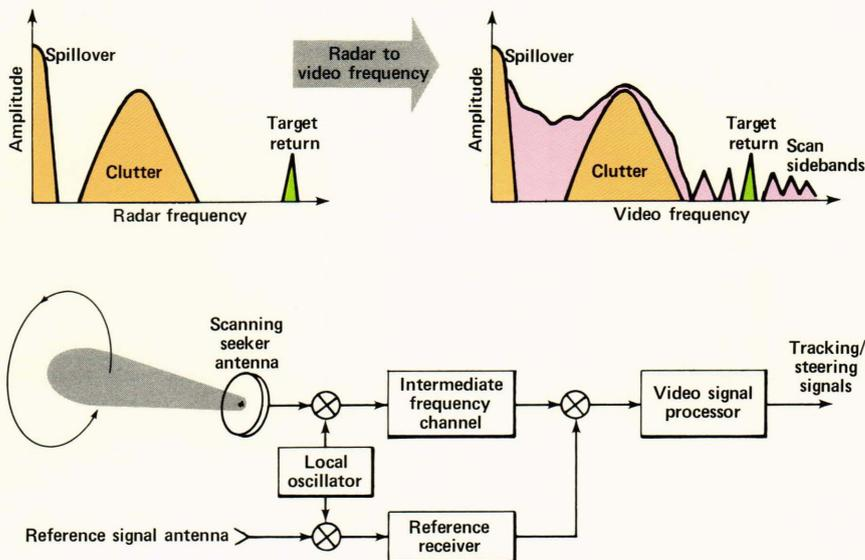
**Figure 7** — Scanning receiver operation. Nutation of the scanning seeker antenna introduces an intentional amplitude modulation on the received signal. The modulation causes sidebands about each return, whether from the target or from clutter. Seeker angle error information is derived from the magnitude of the first scan sideband associated with the target signal. Scan sidebands associated with clutter can interfere with target detection and tracking.
