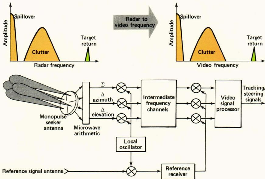
**Figure 8** — Monopulse receiver operation. Angle error information is contained in the relative magnitudes of the  $\Sigma$  and  $\Delta$  signals formed by summing and differencing the signals received by the four symmetrically offset lobes of the monopulse antenna. This simultaneous measurement approach circumvents the amplitude modulation in time-sequential measurement (scanning) receivers, resulting in a significant reduction in Doppler-band interference.
