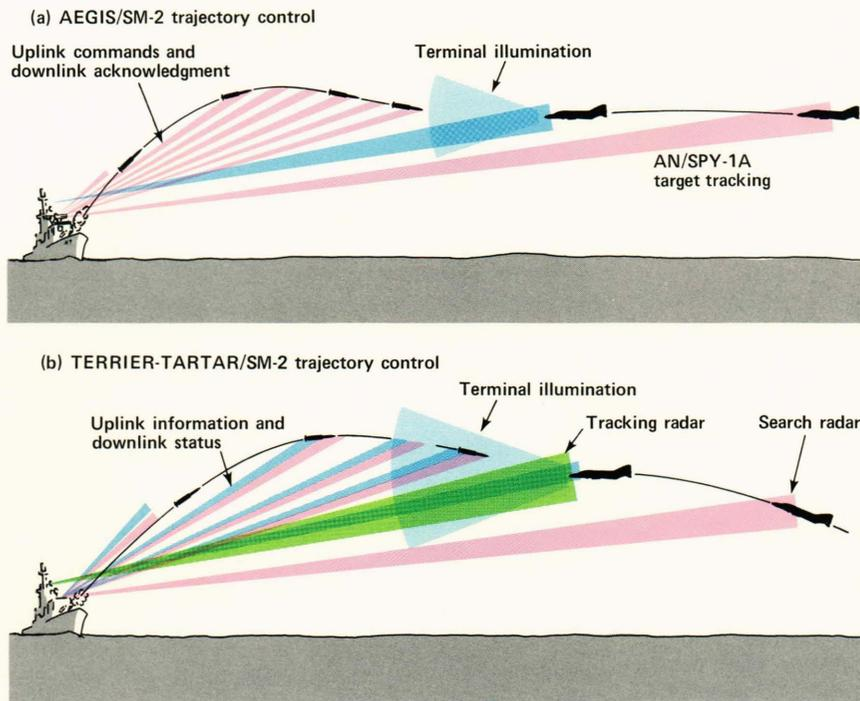
**Figure 5** — SM-2 midcourse plus semiactive terminal guidance. In the AEGIS application (a), SM-2 is guided by the ship through the midcourse phase of flight. Uplink acceleration commands, which are acknowledged via the downlink, are converted into steering signals by the missile inertial reference unit. Terminal homing is commanded by uplink and can be delayed longer than in TERRIER or TARTAR because of greater midcourse accuracy.
