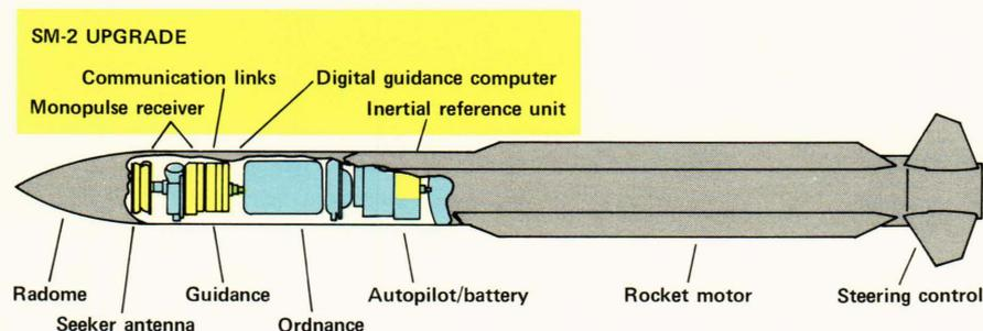
**Figure 1** — STANDARD Missile-1 (SM-1) showing STANDARD Missile-2 (SM-2) additions. Evolutionary improvements to STANDARD Missile have been facilitated by the use of modular packaging. The SM-2 upgrade consisted of a new guidance section and additions to the autopilot/battery section, while other sections remained essentially unchanged.
