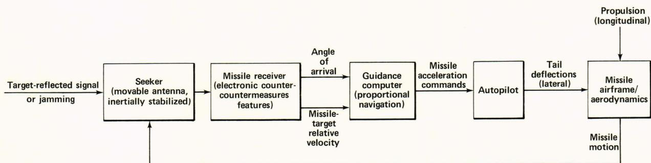
**Figure 6** — Terminal guidance functional block diagram. STANDARD Missile terminal guidance is accomplished by processing an RF signal received from the target. The receiver determines the angle and relative velocity of the target while the guidance computer translates this information into steering commands. The autopilot adjusts the aerodynamic control surfaces to alter the missile's trajectory as required. Kinematic energy is provided by a solid rocket propulsion system.
