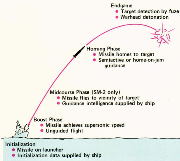
**Figure 3** — STANDARD Missile operational sequence. On the launcher, the SM-1 is supplied with target acquisition data and begins homing shortly after the unguided boost phase of flight. The SM-2, however, undergoes a midcourse phase under ship control; at a predetermined point much later in flight, target acquisition occurs and homing begins. In the endgame phase, the target is detected by a missile-borne proximity fuze and the warhead is detonated close to the target.
