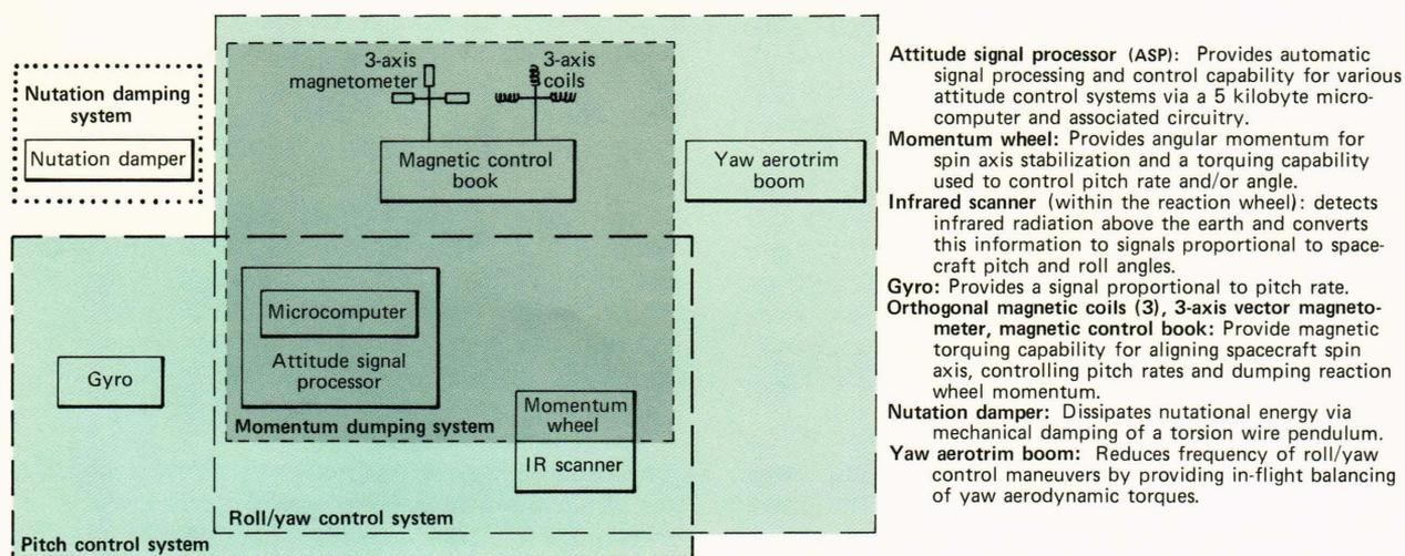
Fig. 1 — Block diagram of the Magsat attitude control system.
