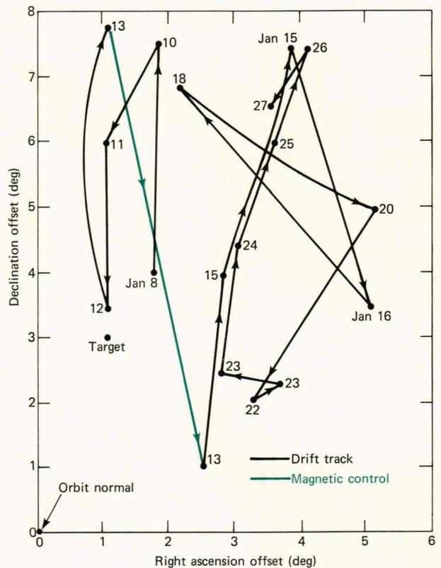
**Fig. 4—Magsat attitude activity from January 8 to 27, 1980, showing drift of the +B axis in space. The roll angle had to exceed a threshold of  $\approx 5^\circ$  (with respect to target position) to initiate roll/yaw control activity. Lack of activity was due to the aerodynamic balancing effect of the yaw trim boom at the skewed target position.**
