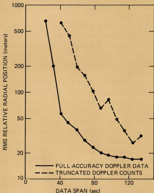
Fig. 10—Observed changes in navigated position versus data span.
