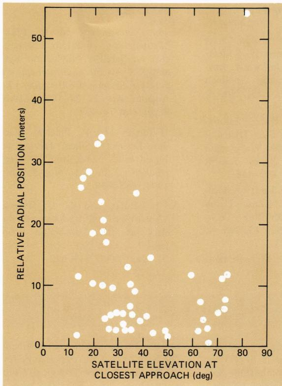
**Fig. 12—Single-frequency (400-MHz) DOPRAN navigated position relative to dual-frequency (150/400-MHz) integral doppler navigated position in 50 passes of the TRIAD satellite at APL.**
