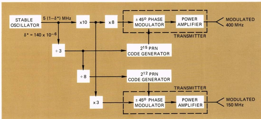
Fig. 1—TRIAD satellite RF system.
