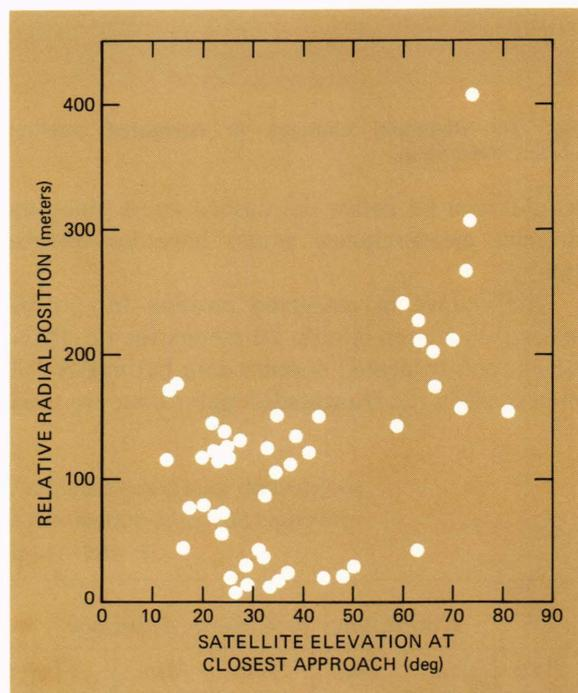
Fig. 11—Single-frequency (400-MHz) integral doppler navigated position relative to dual-frequency (150/400-MHz) integral doppler navigated position in 50 passes of the TRIAD satellite at APL.
