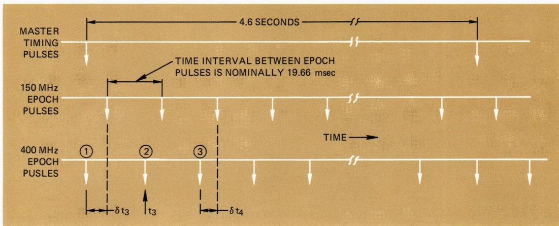
Fig. 7—PRN-ranging measurement timing.
