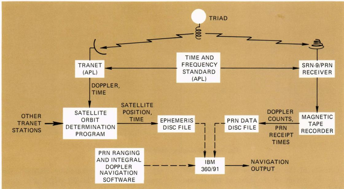
Fig. 8—Elements of the PRN data-gathering system.
