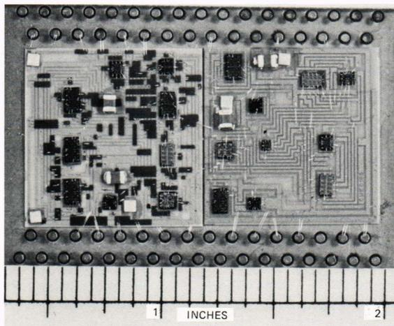
Fig. 2—TRIAD PRN digital generator.
