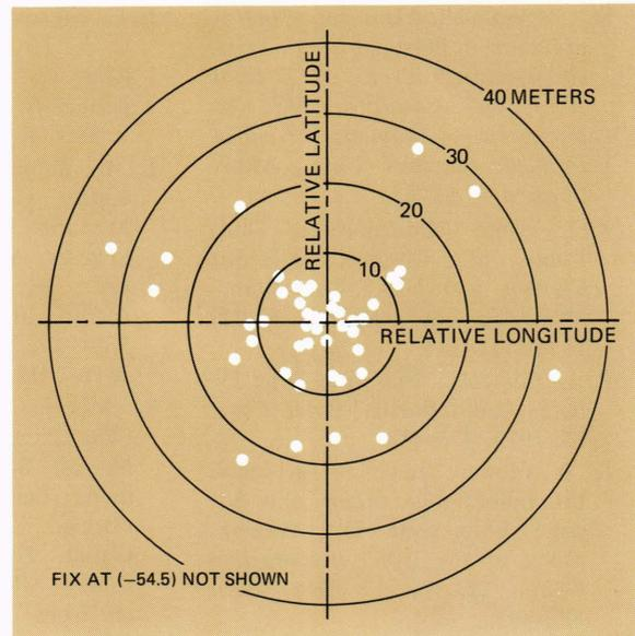
**Fig. 13—Cartesian plot of single-frequency (400-MHz) DOPRAN navigated position relative to dual-frequency (150/400-MHz) integral doppler navigated position in 50 passes of the TRIAD satellite at APL.**
