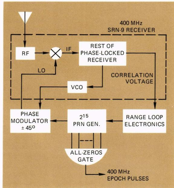
Fig. 5—Modification to SRN-9 400-MHz receiver for PRN signal tracking.
