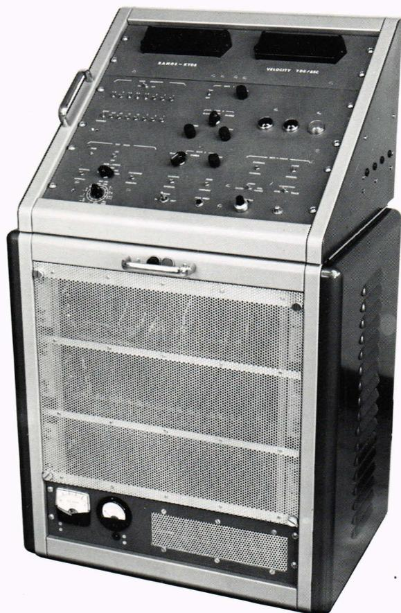
Fig. 1—255:1 digital pulse compression unit and range tracker.
