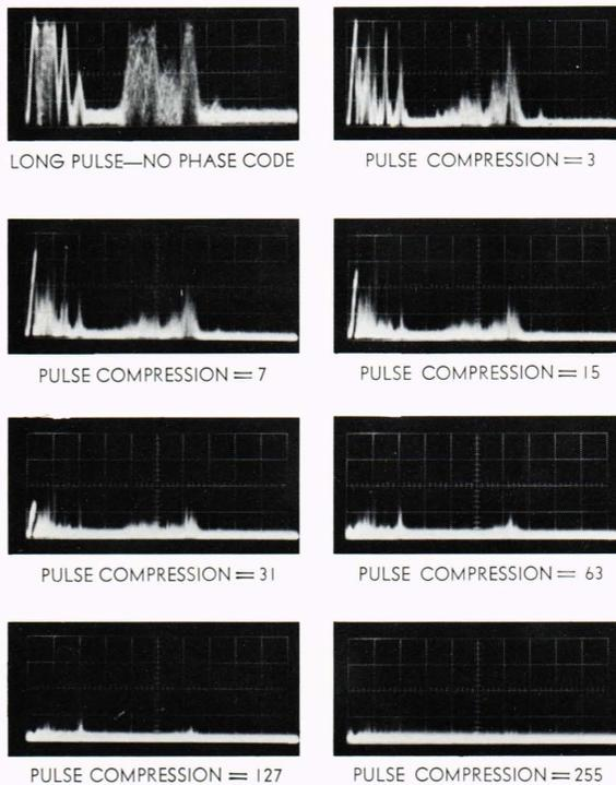
**Fig. 8—Detected video out of digital pulse compressor on rainstorm (100  $\mu\text{sec}/\text{cm}$  common to all).**
