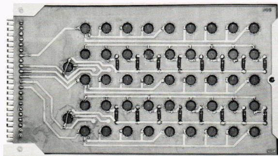
Fig. 3—Eight-stage digital compression card, four-layer board.
