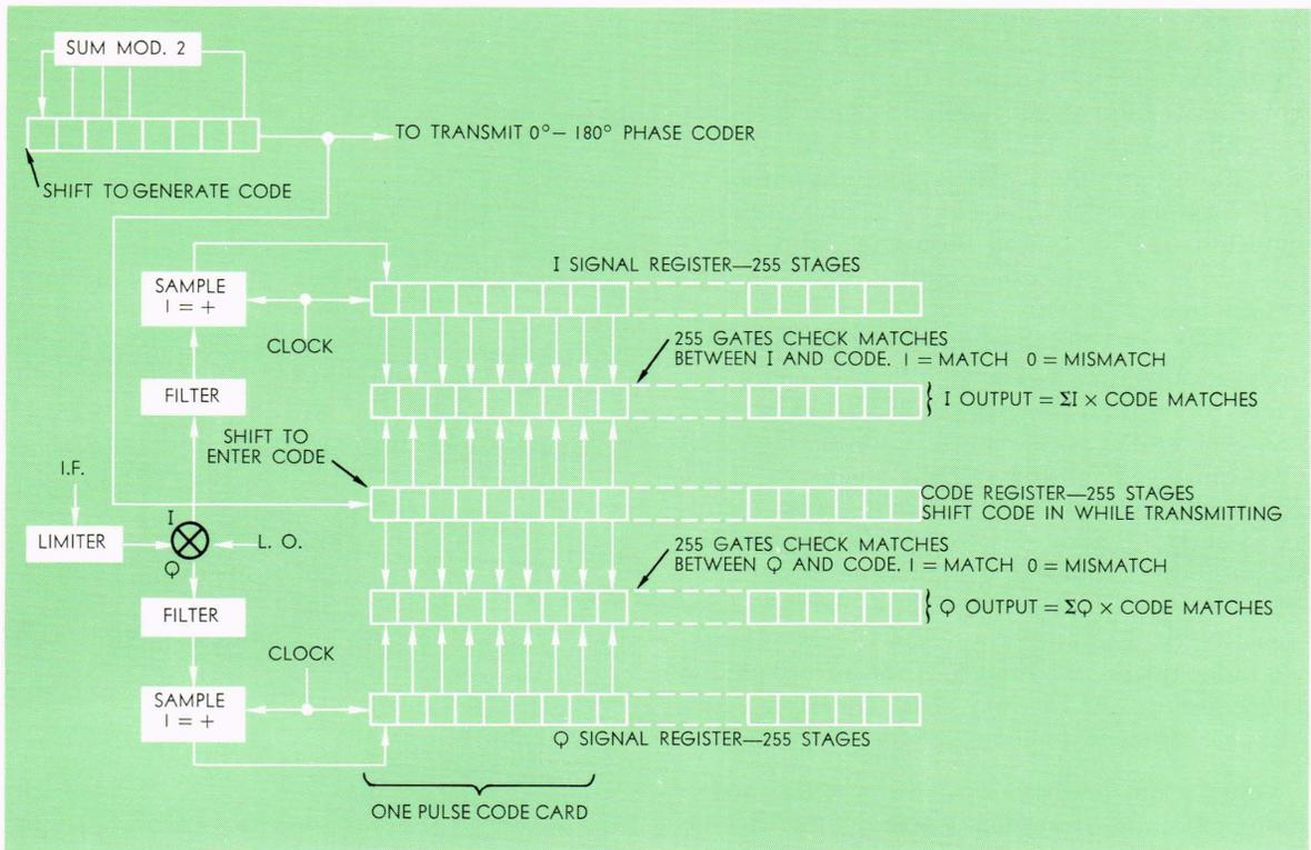
Fig. 2—Block diagram of digital compressor.
