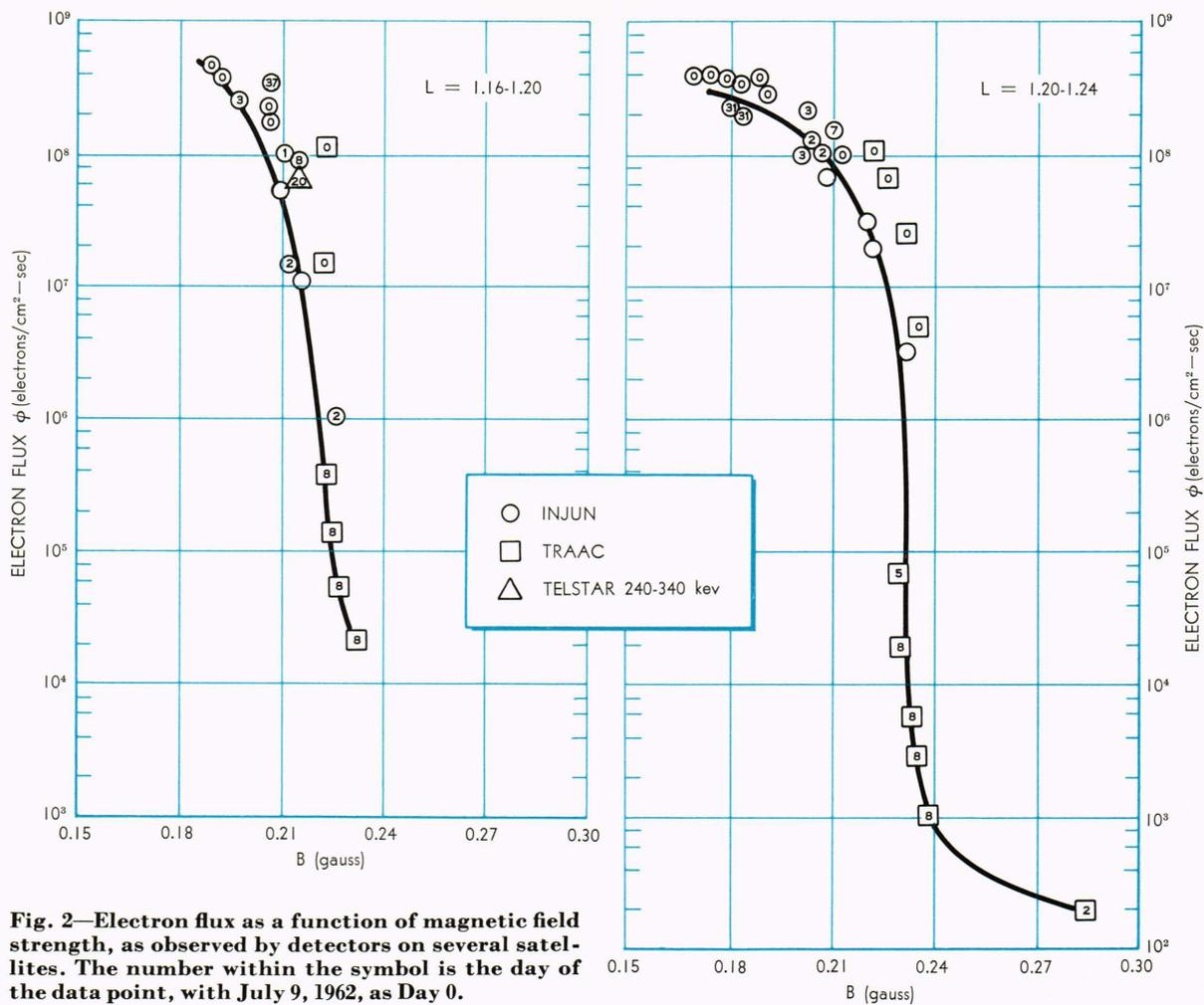
Fig. 2—Electron flux as a function of magnetic field strength, as observed by detectors on several satellites. The number within the symbol is the day of the data point, with July 9, 1962, as Day 0.
