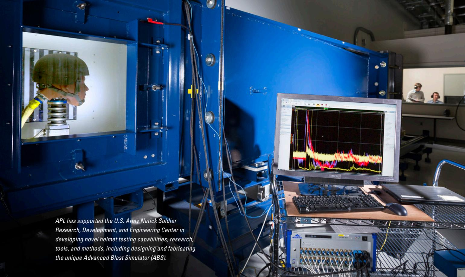
*APL has supported the U.S. Army Natick Soldier Research, Development, and Engineering Center in developing novel helmet testing capabilities, research tools, and methods, including designing and fabricating the unique Advanced Blast Simulator (ABS).*
