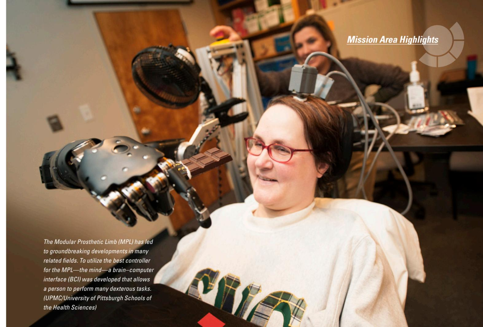
*The Modular Prosthetic Limb (MPL) has led to groundbreaking developments in many related fields. To utilize the best controller for the MPL—the mind—a brain–computer interface (BCI) was developed that allows a person to perform many dexterous tasks. (UPMC/University of Pittsburgh Schools of the Health Sciences)*
