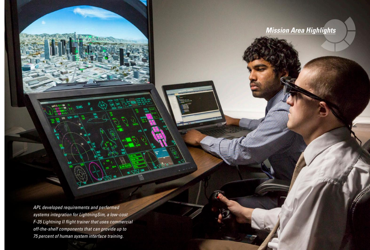
*APL developed requirements and performed systems integration for LightningSim, a low-cost F-35 Lightning II flight trainer that uses commercial off-the-shelf components that can provide up to 75 percent of human system interface training.*
