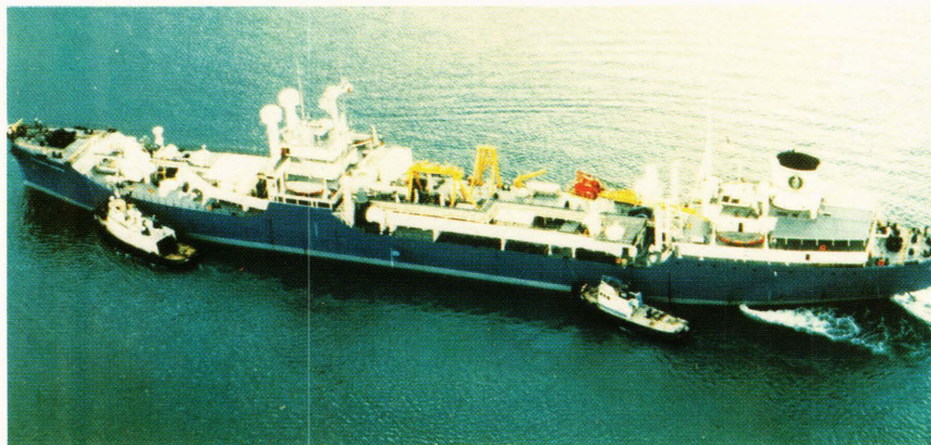
Figure 7 — The OTEC-1 1 megawatt demonstration ship.
