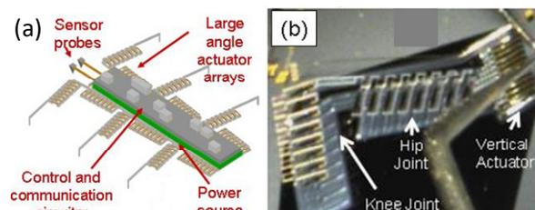
**Figure 1: (a) Concept drawing of an autonomous micro-robot driven by (b) multi-degree-of-freedom piezoelectric leg joints**
