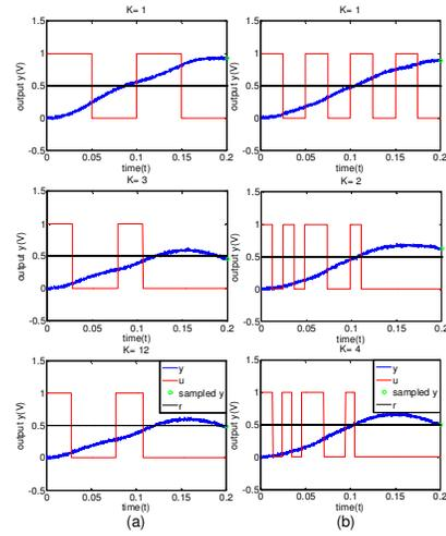
**Figure 3. Output response of the system (17): (a) when  $N = 4$ , (b) when  $N = 8$**
