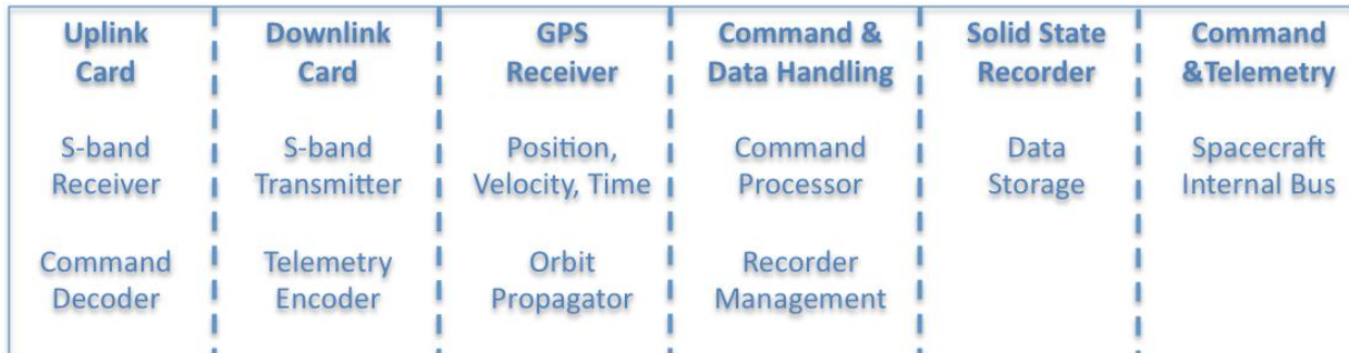
Figure 3 Simplified block diagram of the Integrated Electronics Module of the TIMED spacecraft, showing the on-board GPS Navigation and Orbit Propagation capabilities
