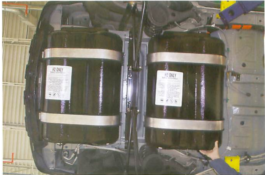
Two APL-patented Integrated Storage Systems are shown installed on the undercarriage of a technology demonstration vehicle.
