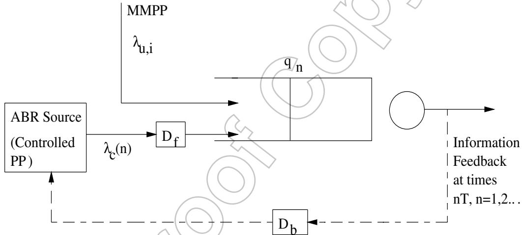
**Figure 8.** The available bit rate (ABR) model
