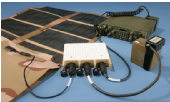
SPACES (Battery Charger)
