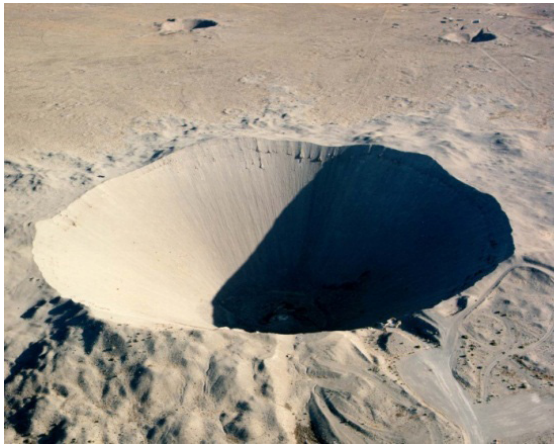
Figure 6.8. The Sedan Crater. A physical relic of the days when the United States and the Soviet Union explored the peaceful uses of nuclear weapons, the Sedan Crater still looms large today at the Nevada National Security Site. Created by a specially designed high-fusion output device with a yield of 104 kilotons detonated at the optimum depth of burst, it is one of the largest such excavations on Earth and served as a training venue for Apollo astronauts. (Image courtesy of the Department of Energy National Nuclear Security Administration/Nevada Field Office.)
