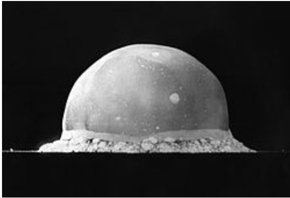
Figure 6.1. Trinity Fireball. As the culmination of the Manhattan Project, the Trinity atomic test was conducted in New Mexico on July 16, 1945. This photograph shows the shape of the fireball, which had a radius of approximately four hundred feet at sixteen milliseconds after detonation. Note the dust skirt traversing the terrain ahead of the main blast wave. 7 (Image courtesy of the Department of Defense.)
