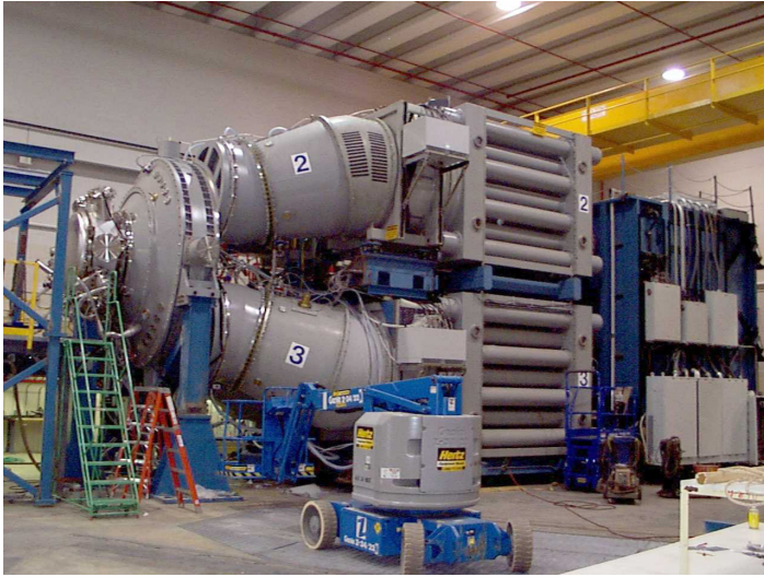
Figure 6.5. DECADE X-Ray Simulator Module. This photograph shows the first of four pulsed power modules planned for the DECADE simulator. The simulator was never completed, a victim of post–Cold War apathy and budgetary declines visited on all matters nuclear. A similar fate eventually befell many other nuclear effects simulators. (Image courtesy of the Department of Defense.)
